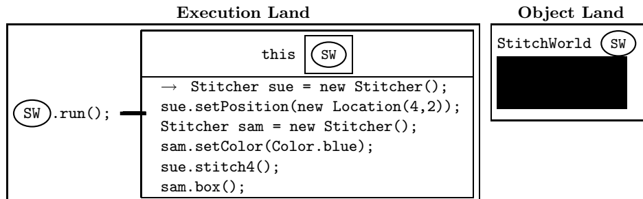
Figure 2: Invoking run() creates an execution frame.
