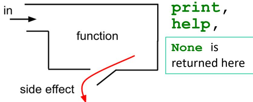
Functions can have **side effects** such as printing (remember, this is not the same as returning). Regardless of whether a function has a side effect, it will always return a value. **None** will be provided as a default. Generally, the function caller will not use the returned **None**. Thus, we write this situation without an out as shown in second picture. The last picture depicts a scenario in which a function has a side effect AND returns a value other than **None**.
